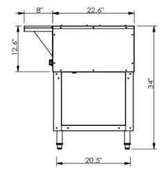
PanUse edgeless water pan.OptionsNoneElectrical120 VoltsPower2000 WattsNet Weight155 lbs.Gross shipping weight170 lbs.Class100Dimensions62.4" W × 30.6" D × 34" HPackage66" W × 26" D × 19" HWarranty1 Year Manufactures limited Warranty
