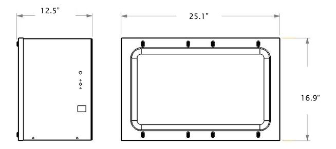
Pan Capacity 20" x 10" x 6" Electrical 120 Volts, 4 Amps,60Hz Power 550 Watts Cord NEMA 5-15P Net Weight 33 lbs(15 Kg) Gross shipping weight 40 lbs(18 Kg) Class 85 Dimensions 25.1" W x 16.9" D x 12.5" H Package 26" W x 17" D x 13.5" H Warranty 1 Year Manufactures limited Warranty
