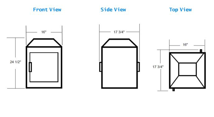
Options None Electrical 120 volts, 60 HZ Power 450 watts Net weight 39 lbs. Gross shipping weight 42 lbs. Class 85 Dimensions 1 6" W X 17.75" DX 24.5" H Package 1 7.75" W X 1 9.75" DX 25" H Warranty1 Year Manufactures limited Warranty
